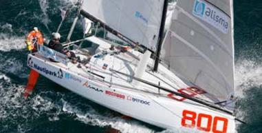
Nautipark (Frederic Denis) wins in the Proto class in 2015. Note the daggerboards, canting keel, chine, flat bottom and twin rudders
