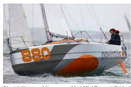
Ofcet 6.50: one of these won 2015 Mini Transat 'Series' production class. The rounded bow and chines contribute to speed and stability
